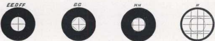
The Sun's disc, as it appears when collimated by Cross-hairs, E, F, G and H in Solar Attachments
