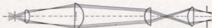
DIAGRAM SHOWING PATH OF A PENCIL OF RAYS IN AN EYEPIECE FOR AN ERECTING TELESCOPE
