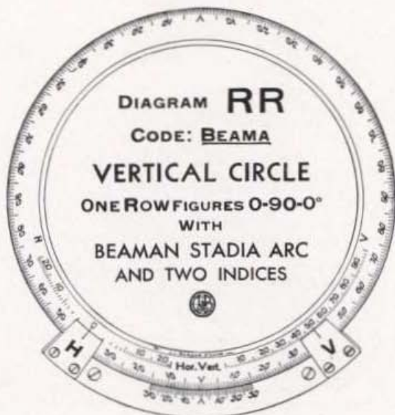
Figuring of Graduations of Vertical Limbs (For a description of the Beaman Arc, see page 18)
